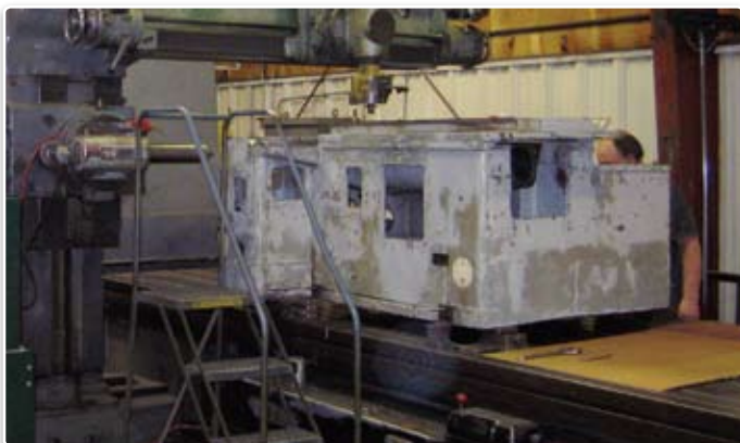
After complete tear down, inspection and evaluation, we grind, scrape and fit all ways.
