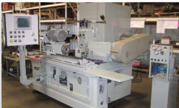
We completely rebuild or install new spindles and make sure that all motors are either rebuilt or replaced. All electric, pneumatic, hydraulic and lubrication systems are replaced with new components.
