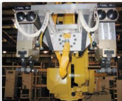
EOAT designed and built for multiple component picking from ID
