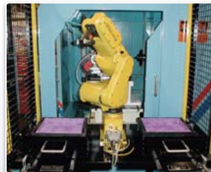
Part picking and placing from removable tray system
