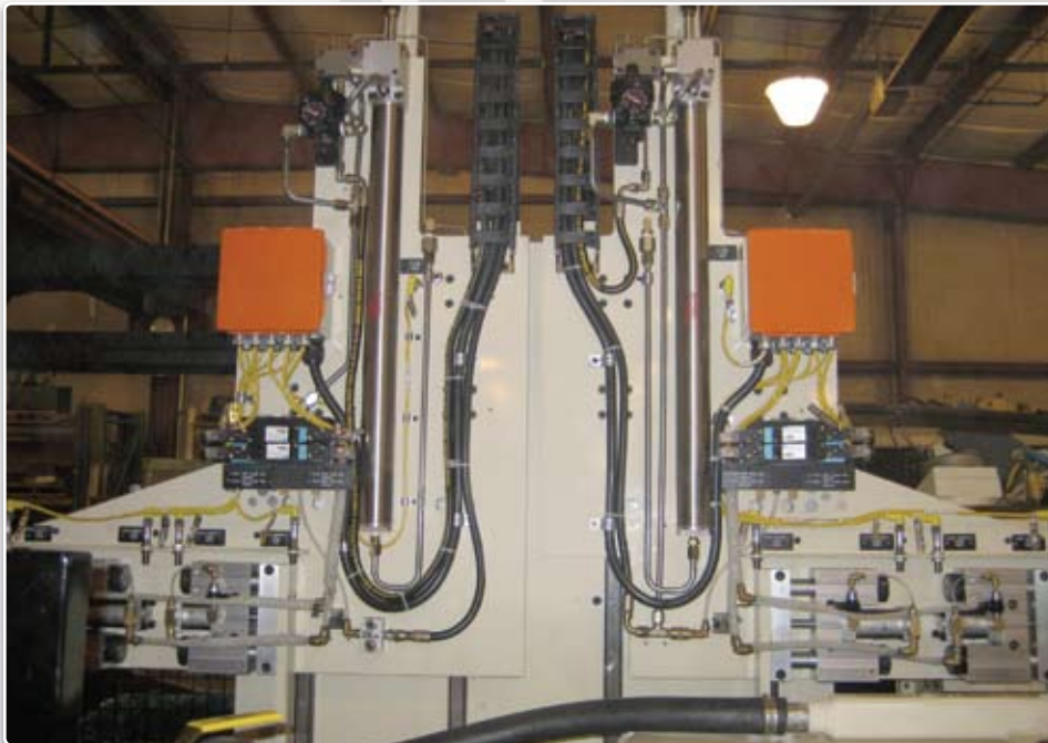
Multi Station loading system with entrance and exit conveyers, fixturing and part paddle stations
