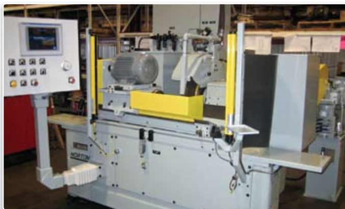
All components are reassembled, mounted and aligned. Machine runoff and quality checks are performed prior to shipment of any completed machine. All rebuilds are performed with safety at the forefront of every project.
