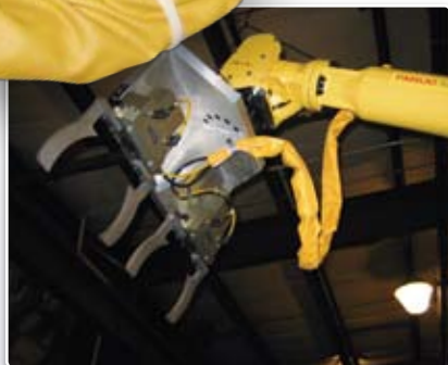
EOAT designed and built for multiple component picking from OD
