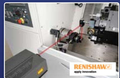
State-of-the-art Renishaw laser performance measurement and calibration systems
